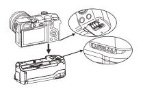
8. Turn the attachment knob to tighten securely. Connect the cable after the battery grip is attached.
