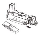
Place the battery holder back into the battery grip and close the control lock by turning the knob clockwise.
